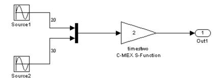
The input to the timestwo S-function comes from two arrays located at two different memory locations, one for the output of source1 and one for the output of block source2. This is because of an optimization that makes the Mux block *virtual*, meaning that code is not explicitly generated for the Mux block and thus processor cycles are not spent evaluating it (i.e., it becomes a pure graphical convenience for the block diagram). So this is represented in the *model*.rtw file in this case as
