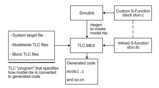
Just as a C program is a collection of ASCII files connected with **#include** statements and object files linked into one binary, a *TLC program* is a collection of ASCII files, also called *scripts*. Because TLC is an interpreted language, there are no object files. The single target file that calls (with the **%include** directive) other target files used for the program is called the *entry point*.
