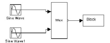
To use ucv in a robust manner, you must use the %roll directive with a roll threshold of 1 and a Roller TLC file that does not have loop header/trailer setup for this input signal. In addition, you need to use ROLL\_ITERATIONS to determine the width of the current roll region, as in the following TLC code:
