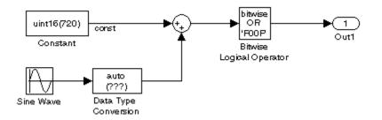
The code generated for the bit-wise operator block reuses a temporary variable that is set up for the output of the sum block to save memory. This results in one very efficient line of code, as seen here.
