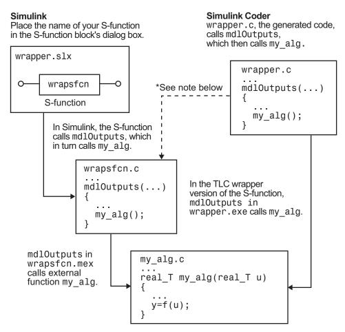
\*The dotted line is the path taken if the S-function does not have a TLC wrapper file. If there is no TLC wrapper file, the generated code calls mdlOutputs.
